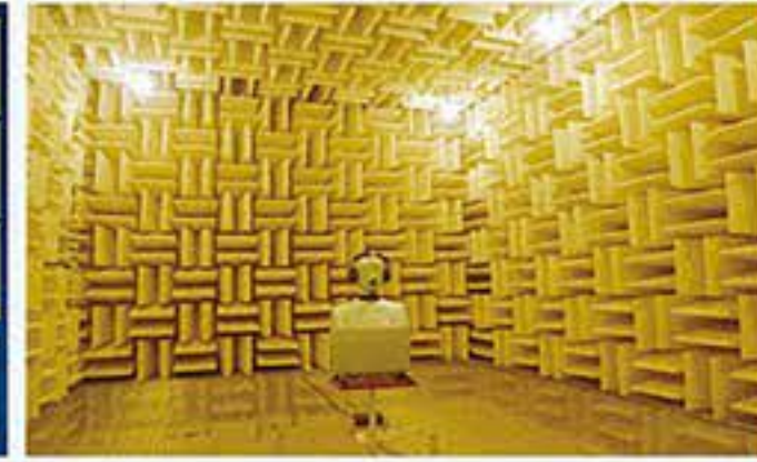
Silencer chamber Noise floor 7.9dB, test frequency range: 50-20KHz
