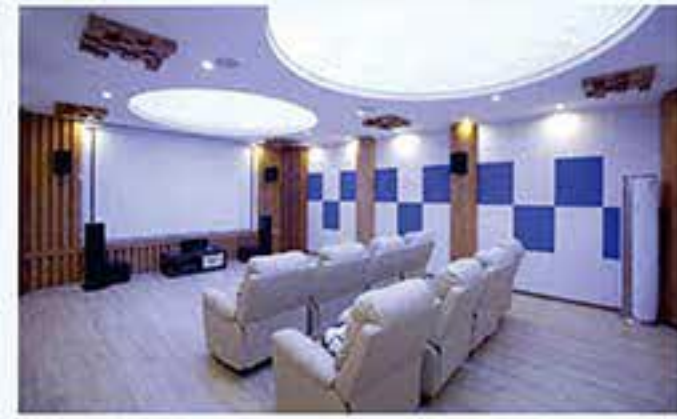
Listening room Noise floor 21.8dB, reverberation time 0.3-0.4s, The test range is 125Hz-8KHz
